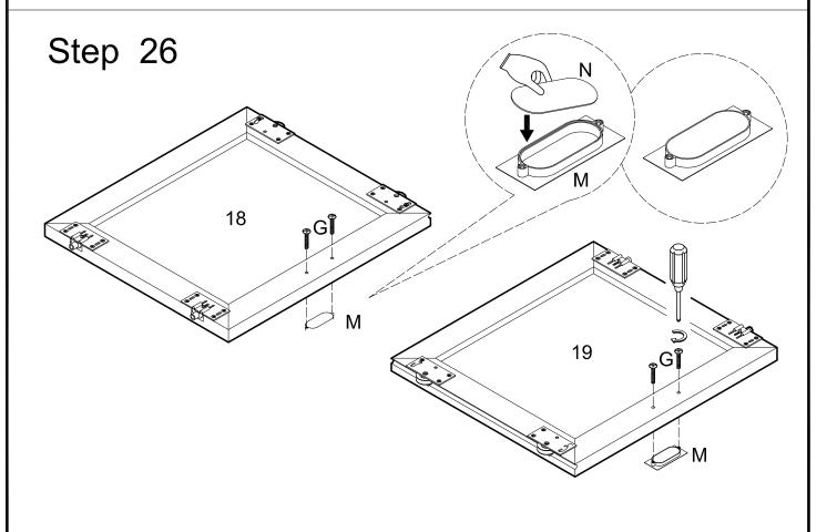
Place the handle back plate (N) into handle (M). Attach the handles (M,N) to doors (18,19) using handle screws (G)
